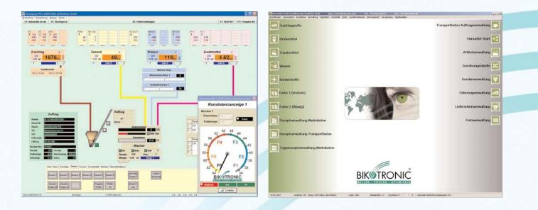
The TB-WIN SQL Process Control System allows the manual and automatic control of the processes in the concrete mixing plant. Thanks to its modular structure a tailor-made plant control can be created. For this, only the hardware and software modules necessary for the specific production process will be compiled.
